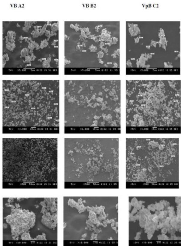
Sample A2 has a particle size ranging from 1.29 µm-5.24 µm while sample B2 with a particle size of 625nm-738nm with few particles ranging from 1.05 µm-2.78 µm. Similarly particle size of the sample C2 ranges from 1.34 µm-4.24 µm.
